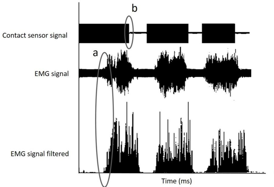
FIGURE 2: EMD detection: a. the onset of the ECR EMG response; b. the first apparent movement the first apparent movement when participants dropped the ball. EMD = time between a and b.
