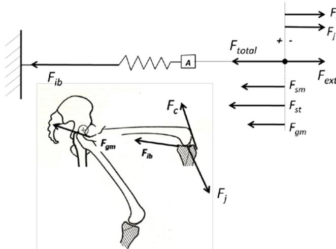
FIGURE 1: Forces applied in the shank during knee extension.
