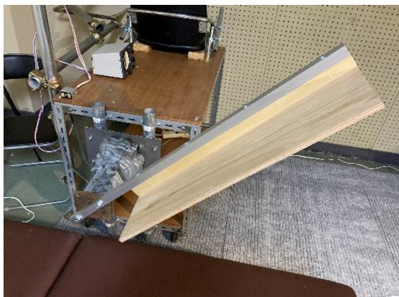
**Figure 1.** Overview of the proprioceptive neuromuscular facilitation (PNF) stretching system developed in this study.
